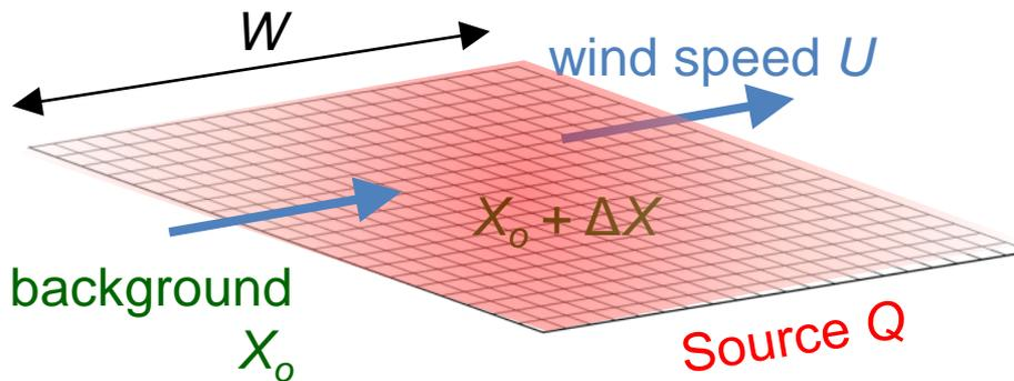
$$t = t_R \max \left[ 1, \frac{1}{FN} \max \left[ 1, \left( \frac{M_{CH_4}}{M_a} \frac{5\sigma U W p}{Qg} \right)^2 \right] \right]$$
