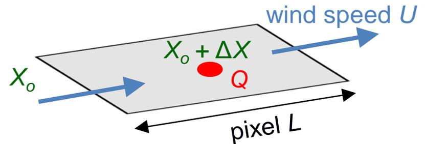
$$Q_{min} = \frac{M_{CH_4}}{M_a} \frac{2ULp\sigma}{g} \sim UL\sigma$$
